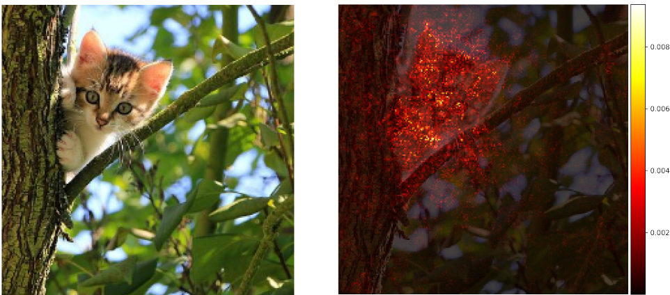
Figure 10.10: An example of a heat map of sensitivity values of an image classification algorithm. As a model we used the pre-trained GoogLeNet [SLJ + 15], which correctly classified the original image (left) as a cat. The sensitivities of the cat class output (right) have been averaged over the three color channels of the input picture. The color represents the magnitude of the sensitivity for each pixel. We see that the pixels which influence the loss the most are indeed the ones showing the cat's shape. (Cat image licensed under Pixabay Content License.)
