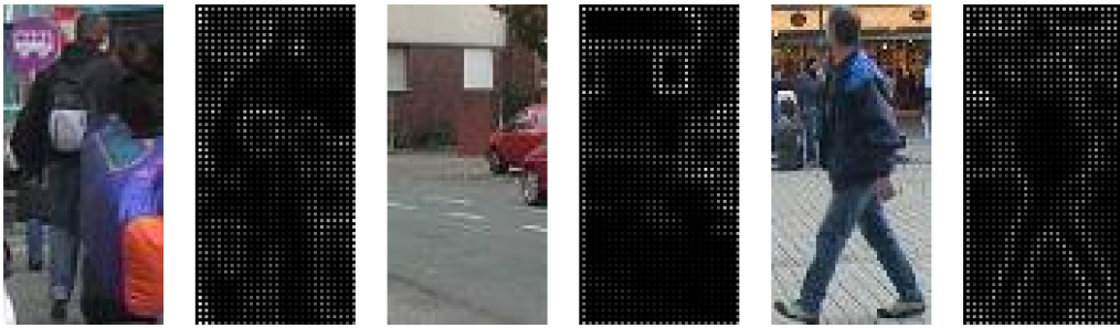
Figure 4.3: Three random images created from the TUD-Brussels data set [WWS09] together with their computed HOG features (right of the respective image). In each (c_y, c_x) -cell of the HOG histogram and for each orientation index b_i we have drawn an arrow with direction corresponding to the orientation from bin b_i . The brightness of each arrow is proportional to the histogram entry H(c_y, c_x, b_i) . To obtain a better visualization we omitted the block building and normalizing steps at the end of Algorithm 4.
