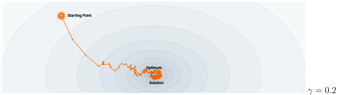
Figure 4.17: For the well-conditioned convex problem, stochastic gradient with constant step size converges quickly to a neighborhood of the optimum, but then bounces around.
