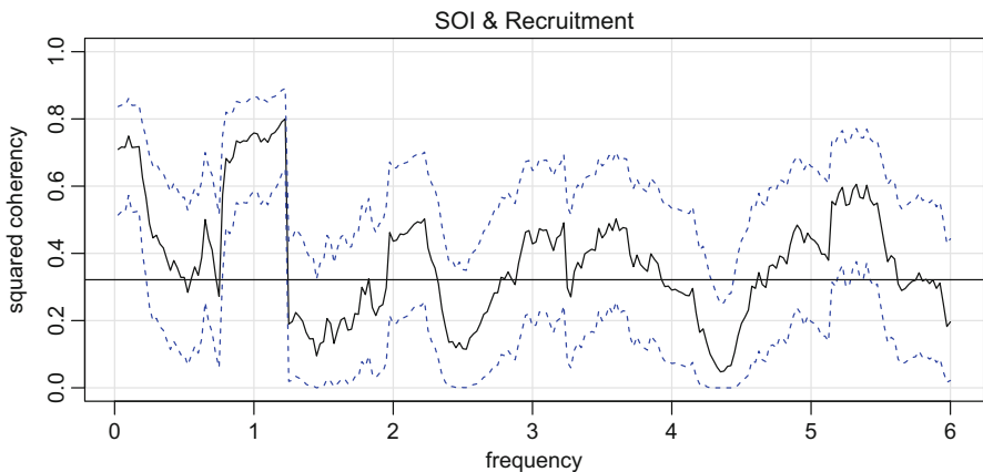
Fig. 4.15. Squared coherency between the SOI and Recruitment series; L = 19 , n = 453 , n' = 480 , and \alpha = .001 . The horizontal line is C_{.001}
